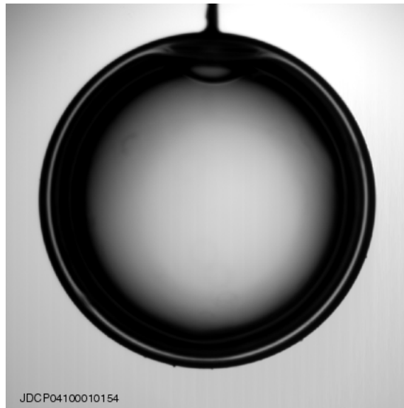
Figure 4-5. Cryogenic layering experiments at LLNL have demonstrated cryogenic hydrogen ice layers that meet the NIF ignition requirements for temperature and smoothness. The figure shows a 1 mm diameter polymer capsule containing a 100- \mu\text{m} thick layer of HD ice that has been layered and smoothed by illumination with infrared laser light. The outside of the thin "bright band" images the ice surface and shows an rms roughness of 0.7 \mu\text{m} (modes 3-100) at a temperature 1.5 K below the melting point, as specified for the NIF ignition targets.
