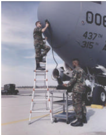
Mobile Automated Scanner Nondestructive Evaluation System
